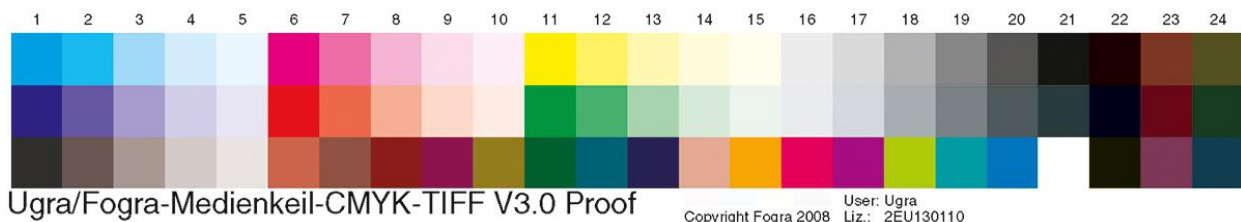
Figure 1. UGRA/FOGRA MediaWedge v.3.0 control scale.
